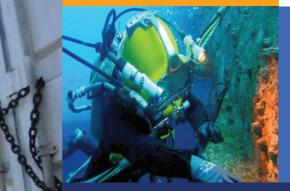
A ship's hydrodynamic performance can be adversely affected by the accumulation of marine detritus. This can not only result in decreased speed and power performance, but an increase in fuel consumption, and hence cost. Regular cleaning of the hull can prevent fouling as well as the spread of potentially invasive species. Through the use of our tried-and-tested cleaning systems, we can ensure a thorough clean, with no damage done to the paint work.
