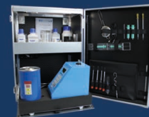
"FUEL AND LUBE OIL TEST CABINET"
